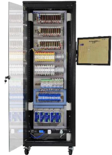
**PLC Control Function based on IEC61131-3**
